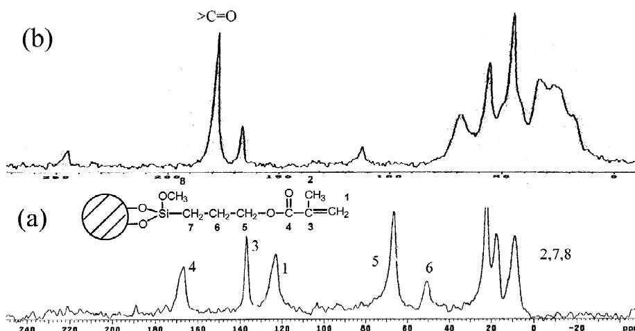
Fig. 4. Solid state  $^{13}\text{C}$  NMR for the polymeric stationary phase with DETA. (a) Vinyl group-modified silica gel and (b) polymeric stationary phase with DETA.
