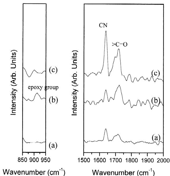
Fig. 3. FT-Raman spectra for the polymeric stationary phase with DETA in the 850–950 and 1500–2000  $\text{cm}^{-1}$  regions. (a) Vinyl group modified silica gel, (b) GMA-modified silica gel, and (c) polymeric stationary phase with DETA.
