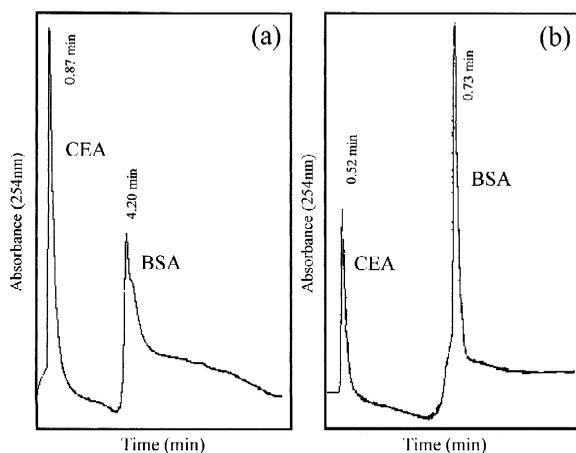
Fig. 6. Separation of CEA and BSA using the EDA column (a) and DETA column (b). Mobile phase: buffer A: Tris–HCl, pH 7.4; buffer B: 1.0 M NaCl.
