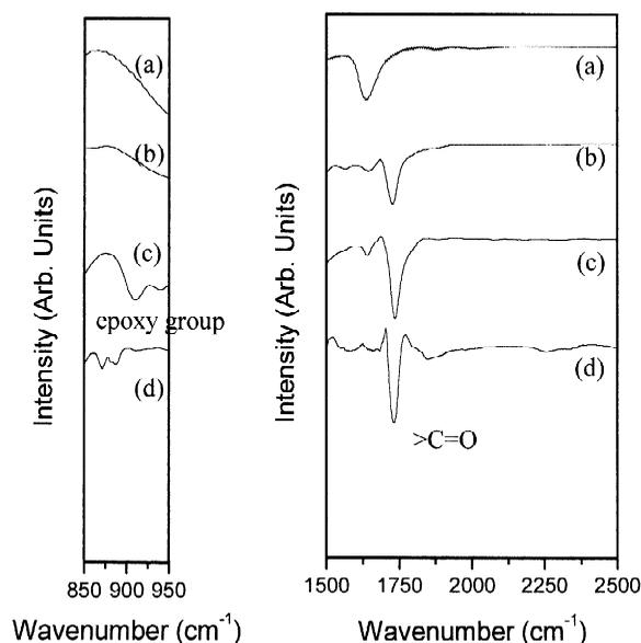
Fig. 2. FT-IR spectra for the polymeric stationary phase with DETA, in the 850–950 and 1500–2500  $\text{cm}^{-1}$  regions. (a) Silica gel, (b) vinyl group-modified silica gel, (c) GMA-modified silica gel, and (d) polymeric stationary phase with DETA.
